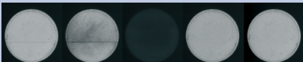
transition from a supercritical monophasic state (2 images on the left) to a liquid-vapour state (2 images on the right), presence of an interface.
